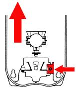
To release valve, push in side catch & lift valve upwards.
